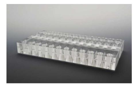
Consists of a clear polyacril block with 12× extra strong permanent magnets for a fast magnetic separation with 1.5 ml and 2.0 ml tubes.
