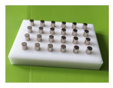
Consists of a polyacetal (POM) block with 6 x 4 extra strong permanent magnets (d = 7.5 mm) for fast magnetic separation with 96 well plates.
