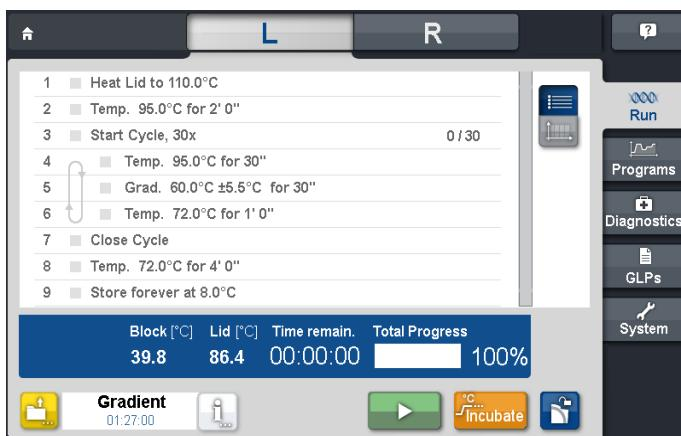
Note: At peqSTAR 2X double block thermal cyclers the desired block can be chosen in the dialogues 'L' (left) and 'R' (right). For peqSTAR XS, 96X, 384X and in Situ X systems this option is not available.
