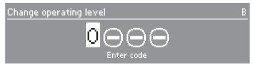
The ▲ ▼ buttons alter the values, the **OK** button confirms the values entered and moves on to the next input position.
