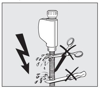
The inlet hoses must **not** be shortened or damaged in any way (see illustration).
