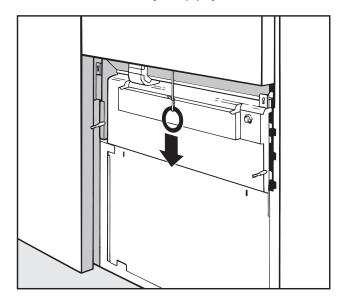
■ The emergency release cable is located at the bottom of the machine behind the service panel. Pull it downwards to open the door.
