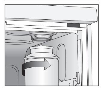
■ Screw the salt container firmly onto the socket.
