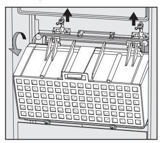
■ Remove the coarse filter housing.
