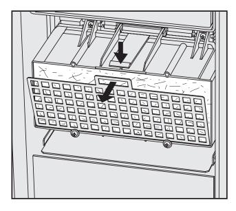
■ Remove the filter grille from the drying unit.
