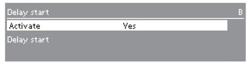
■ To set the Delay start time, highlight the **Delay start** parameter and confirm your selection.
