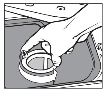
■ To unscrew the micro-fine filter, take hold of the two lugs and turn twice in an anti-clockwise direction.
