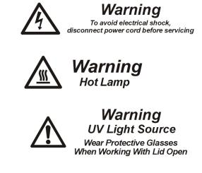
Figure 4 Warnings on the inside of the lamp compartment
