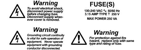
Figure 2 Warning labels on the rear of the instrument
