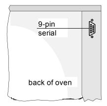
A **serial interface** located on the back panel of the cabinet (see illustration) is provided to link your Type E cabinet to the PC.
