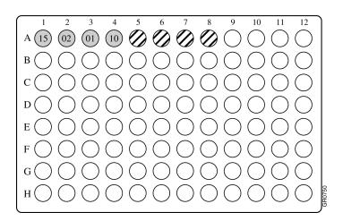
**Figure 3-9** Kit B pooled PCR products in positions A1 through A4. Matrix standard samples in positions A5 through A8.
