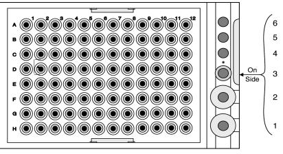
Figure 4-3 Autosampler tray numbering (96 tube positions)
