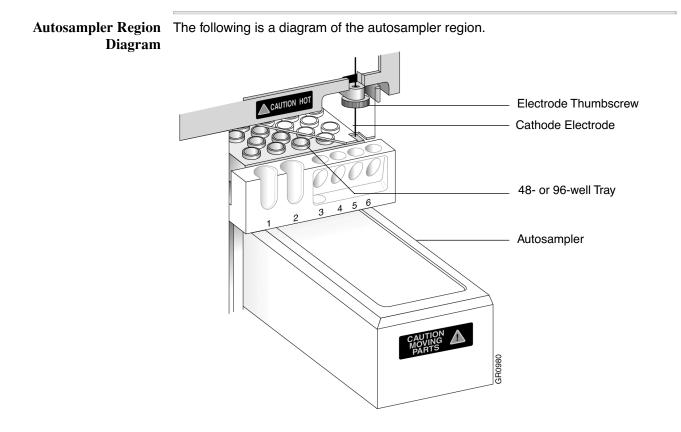
Autosampler Region The following table lists the parts to the above diagram. The autosampler moves Diagram Described buffers and samples to the capillary.
