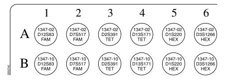
Figure 3-3 Control DNA and primer mix loading diagram for Kit A
