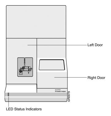
Led Status The LED Status Indicators are red, amber, and green lights. The pattern of lights indicators indicates the instrument's state.
