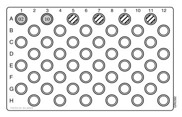
**Figure 3-6** Kit A pooled PCR products in positions A1 and A3. Matrix standard samples in positions A5, A7, A9 and A11.
