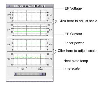
The amps, volts, laser mW, and temperature scales are adjustable. The pop-up windows for adjusting scale overlay the history window, and all four are identical.
