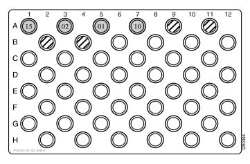
**Figure 3-7** Kit B pooled PCR products in positions A1, A3, A5 and A7. Matrix standard samples in positions A9, A11, B2 and B4.
