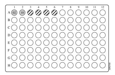
**Figure 3-8** Kit A pooled PCR products in positions A1 and A2. Matrix standard samples in positions A3 through A6.
