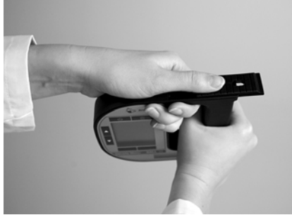
Fig. 11 - 3 Removing the pump lock
