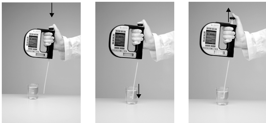
Fig. 9 - 1 Filling sample using the filling tube
