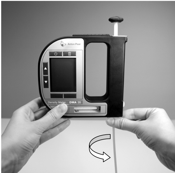
Fig. 7 - 1 Connecting the filling tube
