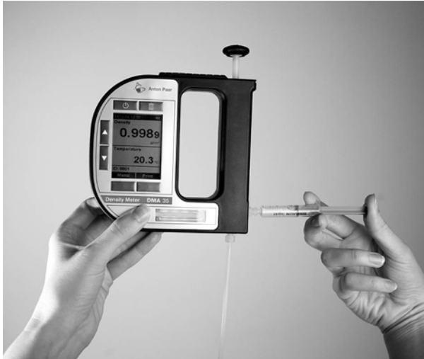
Fig. 9 - 2 Filling sample using the plastic syringe
